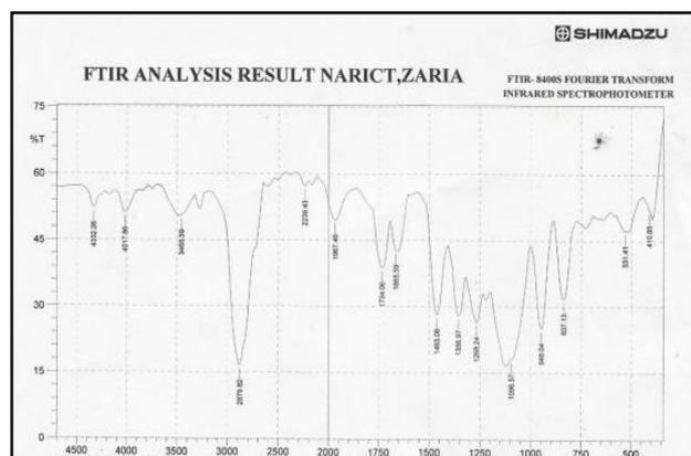
Figure 7: FT-IR spectrum of batch F-3
