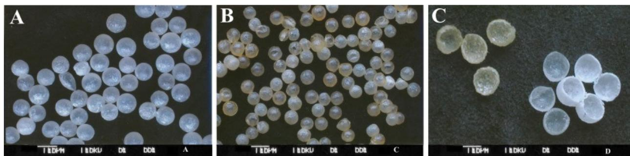
**Figure 1:** SEM image of indomethacin microballoons with (A) coat: core ratio of 2:1, (B) coat: core ratio of 1:3 and (C) inside view.
