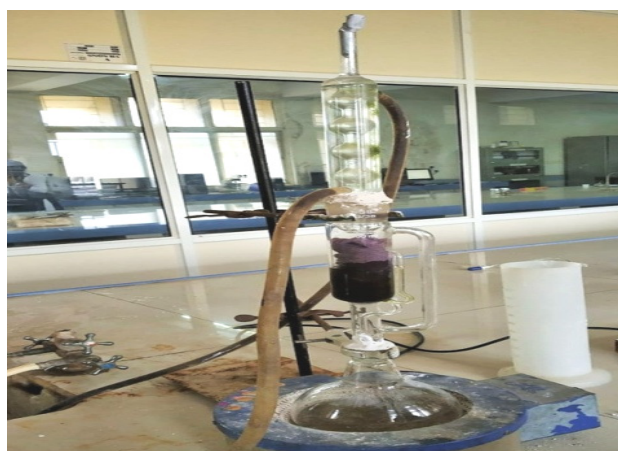
Figure 1: Soxhlet extraction of Acacia arabica L. Pods
